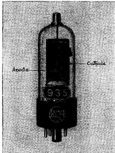
photosensitive materials mentioned above, is a section of a cylinder, while the anode is in the form of a rod, as shown in Fig. 15-46. Light energy enters the glass envelope and strikes the photosensitive surface.
