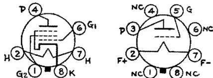
pentode wherein prongs 3 and 5 are eliminated from the base and Fig. 15-2 shows all the eight prongs on the base, but numbers 1, 4, 6, and 8 are unused, being marked "NC" meaning no connection.
