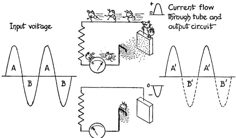
Plate current flows during positive alternation and plate is positive with respect to cathode. Plate current does not flow when plate is negative with respect to the cathode. Thus output current and voltage is unidirectional although input is alternating.
