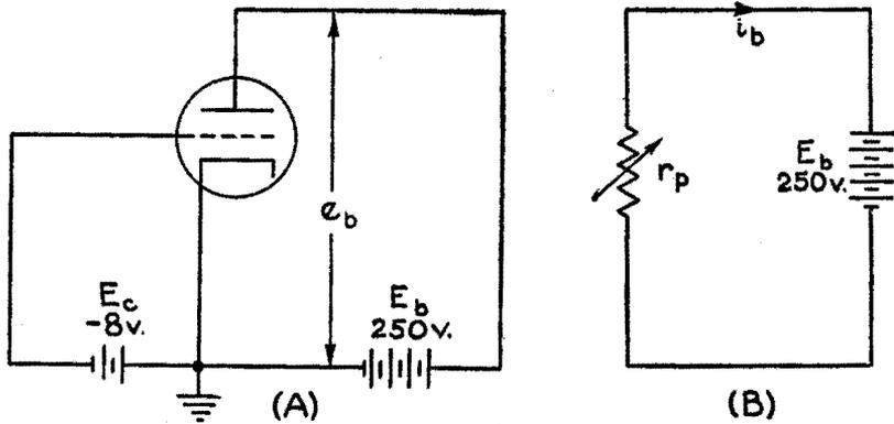
FIG. 9-2. The triode circuit in (A) has no load resistance in the plate circuit ( $R_b = 0$ ) and no input signal; compare Fig. 9-1. The equivalent circuit of (A) is shown in (B) where the plate resistance  $r_p$  is shown as a variable resistor.
