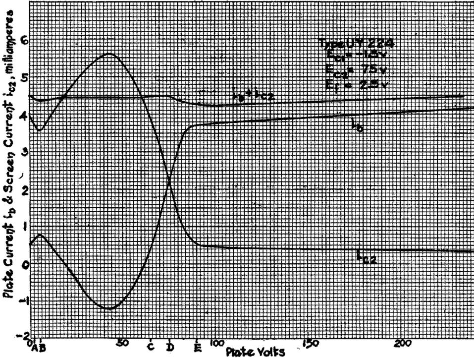
FIG. 12-6. The plate voltage—plate current characteristic curves showing the variations of current flow in the plate and screen-grid circuits, (curves marked  $i_b$  and  $i_{s2}$  respectively) and the total current flow, which is the sum of these two currents.
