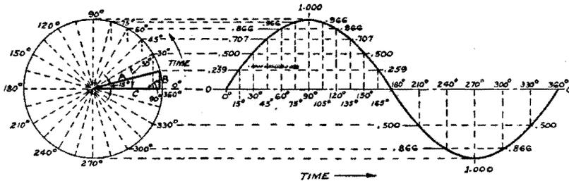
FIG. 10-7. The instantaneous values of a sine wave for every  $15^\circ$  are shown at each division of the positive half-cycle; although not shown in entirety, these values are the same for the negative half-cycle.
