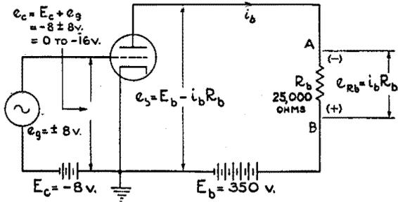
Fig. 9-1. The basic circuit for explaining the dynamic characteristics of a triode. The various symbols are explained in the accompanying text.
