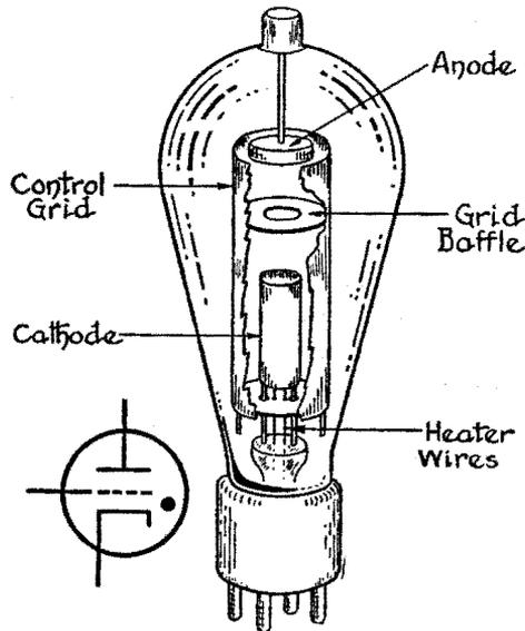
which is part of the grid structure and is called the *grid baffle*. These electrodes are connected to prongs on the base of the tube in the usual manner. The anode consists of a thicker disc than the grid baffle and is connected to the external circuit by a terminal cap on the top of the glass envelope. The grid extends above the anode and below the cathode in order to shield the so-called *discharge path* from charges
