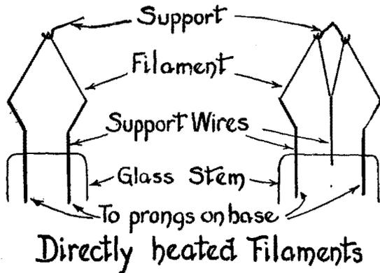
form of an inverted V or W, being mounted and held in place by suitable metal supports which rest in the glass stem of the tube. The filament voltage is applied across the prong terminals of the filament in the tube base and the current flowing in the filament heats it to the electron-emitting temperature.
