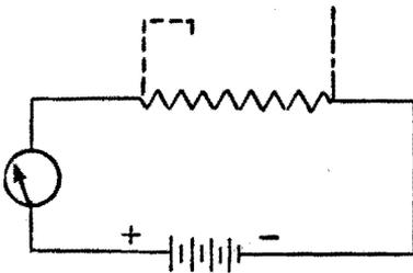
FIG. 7-12 (left). A negative grid bias is the equivalent of a very high resistance between the cathode and grid that prevents any current flow.
