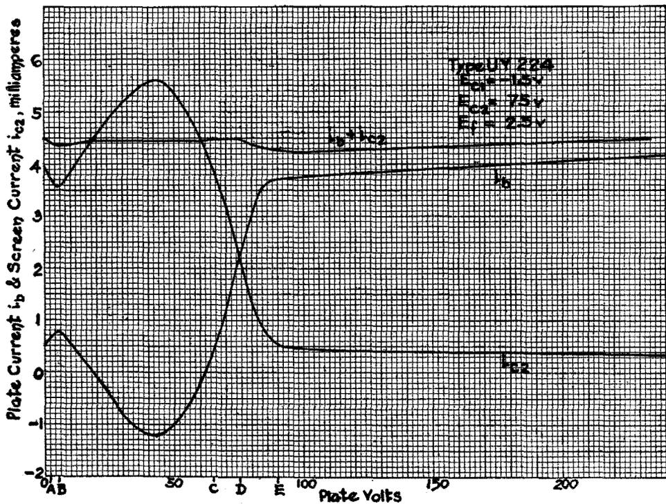
FIG. 12-6. The plate voltage—plate current characteristic curves showing the variations of current flow in the plate and screen-grid circuits, (curves marked  $i_b$  and  $i_{c2}$  respectively) and the total current flow, which is the sum of these two currents.
