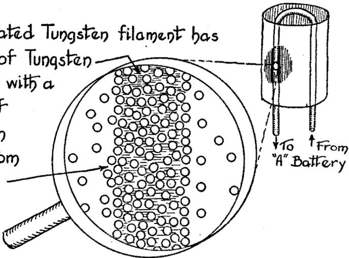
Thoriated-tungsten filaments as electron emitters largely supplanted tungsten filaments in receiving and low-powered transmitting tubes. This type of filament affords the advantage of greater electron emis-
