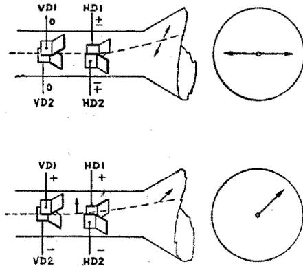
cated in the circle of Fig. 15-33. If the two voltages had been unequal but with the polarities the same, then the spot would have moved at some other angle, depending on which voltage was the greater.
