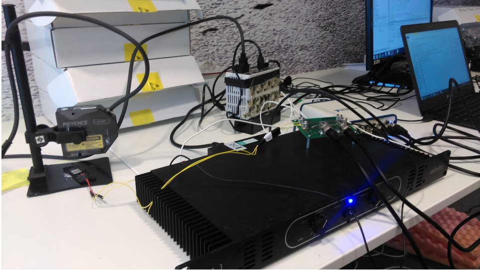
Figure A.1: The experimental setup used in this thesis. The speaker is situated on the left and measured by the laser. The amplifier and the circuit board is situated in the middle. The I/O device and the computer that collects the measurements can be seen to the right.
